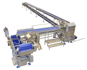
The line for apple processing combines existing machines from different manufacturers with new machines and conveyor belts
