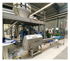
The processing line, besides the washing machines, includesa GS 10-2 belt cutting machine as well as a packaging system.
