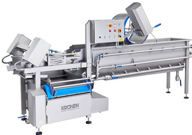
A washing machine, e.g. the GEWA 3800V PLUS, is used to Wash various types of vegetables before further processing.
