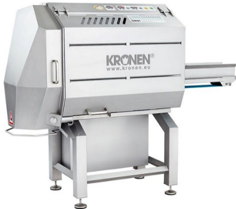
The belt cutting machine GS 10-2 can be used for different cuts by changing the settings and the blade.
