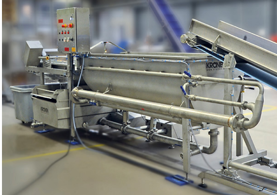
The GEWA 4000V RT, here integrated in a processing line, ensures an efficient washing process
