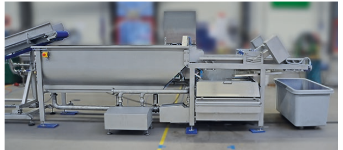
Thanks to adjustable retention time and weighing of products when filling the machine, an optimal washing result is ensured.
