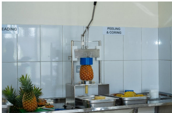
Left: The AS 1 grid cutter for peeling and coring the pineapples at the production facility, which was installed by Twiga Sun Fruits in the Ugandan sub-county of Kangulumira for a smallholders' cooperative.
