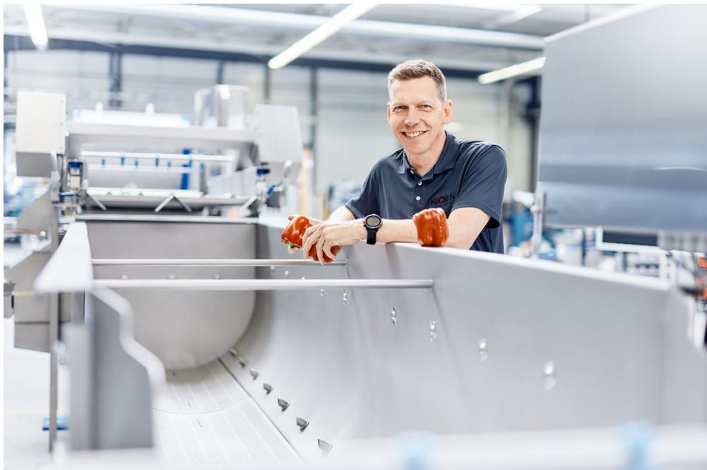
The HEWA 3800 HELICAL washing machine for lettuce, fruit, vegetables, herbs and other foods has been optimized in terms of hygiene and easy cleaning. The design concept also ensures maximum hygiene, for example the fact that the machine has no horizontal surfaces whatsoever, thus allowing the water to optimally discharge. What's more, all edges are designed to avoid the formation of biofilm.
