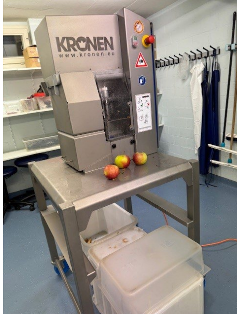
The AS 6 apple peeling machine from KRONEN simplifies apple processing at the Kartause Ittingen Foundation.
