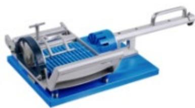
The MMC 150 is a solution in the field of manual tabletop devices. The manual melon chunk cutter can be used to quickly and easily cut prepared melons into slices and segments at the same time.
