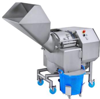
In addition to many other well-established machines, the demonstrations will also feature the KUJ HC-220 cube, strip & slice cutting machine, which can cut large quantities of fruit, vegetables, and other foods with a capacity of up to 8,000 kg/h. The machine also processes large products with a diameter of up to 220 mm with the highest cutting quality.
